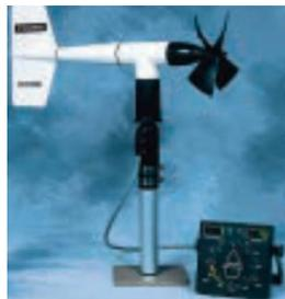
The instrument is made of UV stabilized plastic with stainless steel and anodized aluminum fittings. Precision grade, stainless steel ball bearings are used. Transient protection and cable terminations are in a convenient junction box. The instrument mounts on standard 1 inch pipe.
