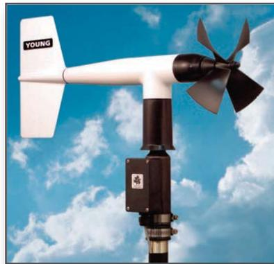
The wind direction sensor is a rugged yet lightweight vane with a sufficiently low aspect ratio to assure good fidelity in fluctuating wind conditions. Vane angle is sensed by a precision potentiometer housed in a sealed chamber. With a known excitation voltage applied to the potentiometer, the output voltage is directly proportional to vane angle. A mounting orientation ring assures correct realignment of the wind direction reference when the instrument is removed for maintenance.
